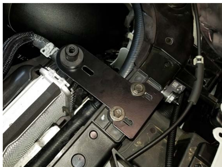
Radiator Bracket Installed
