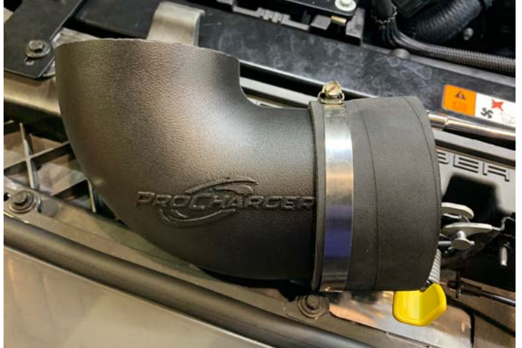
Plastic Inlet Installed
