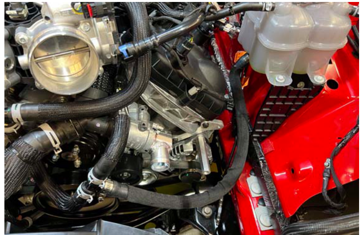
Coolant Hose Installed
