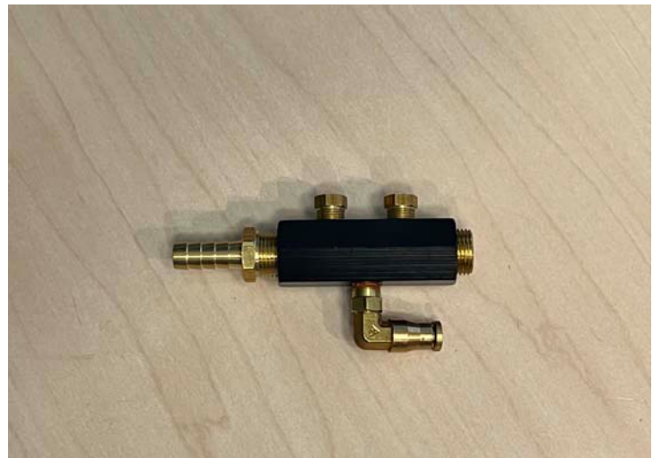
Vacuum Manifold Assembled
