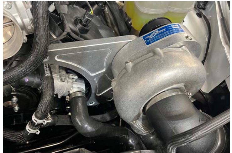
Supercharger And Bracket Installed
