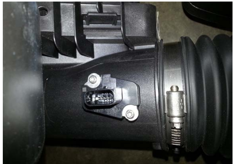
MAF in Factory Air Inlet
