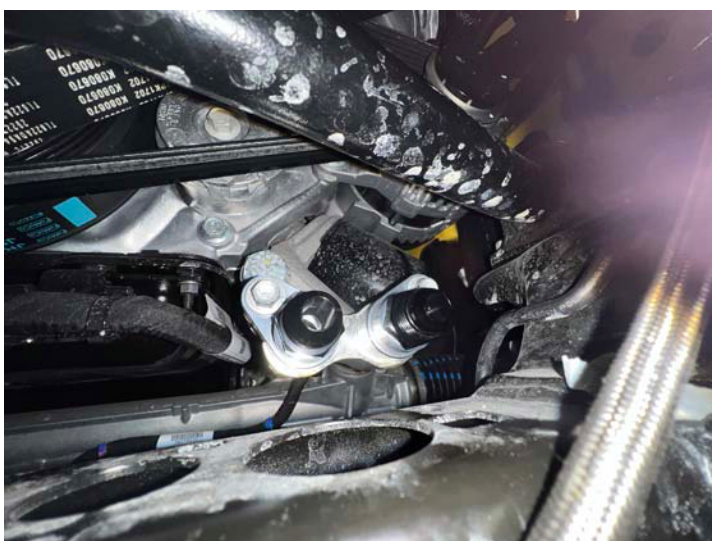
Oil Cooler Adapters Installed
