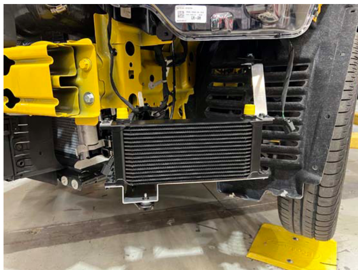
Oil Cooler Installed
