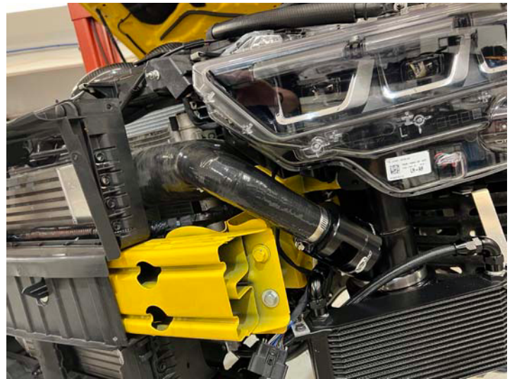
Surge Valve Installed
