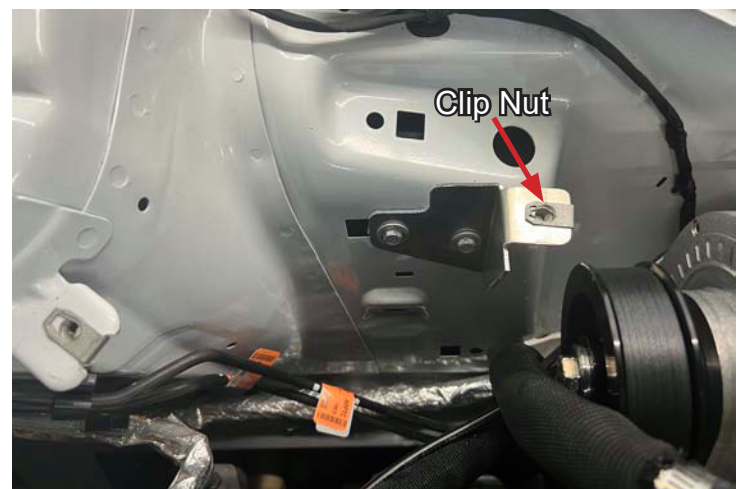
Coolant Tank Bracket Installed
