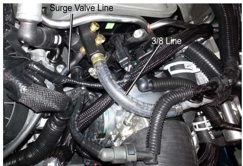
Vacuum Manifold Installed
