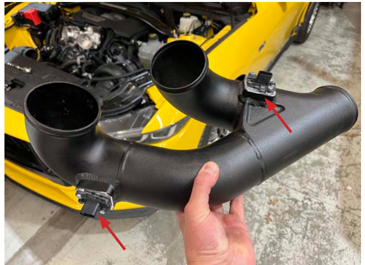
MAF Sensors Installed
