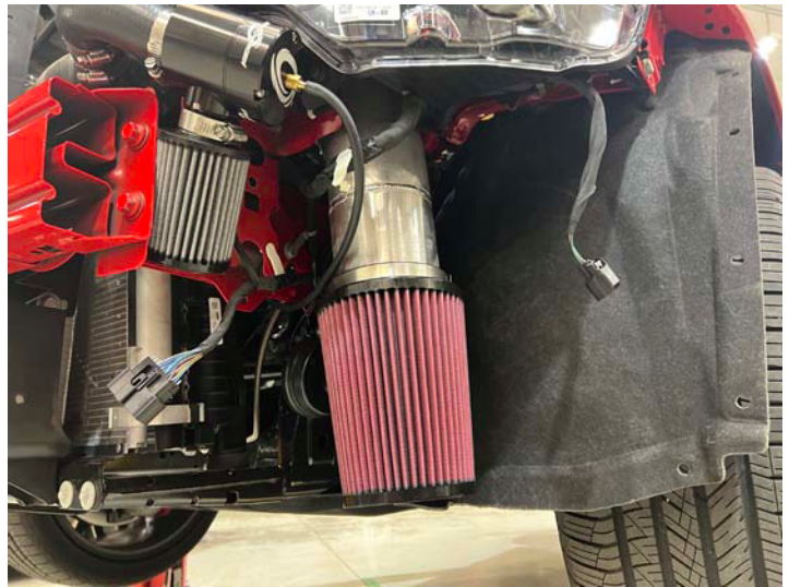
Air Inlet Installed
