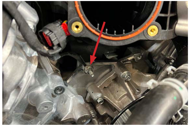
Ground Wire Installed On stud
