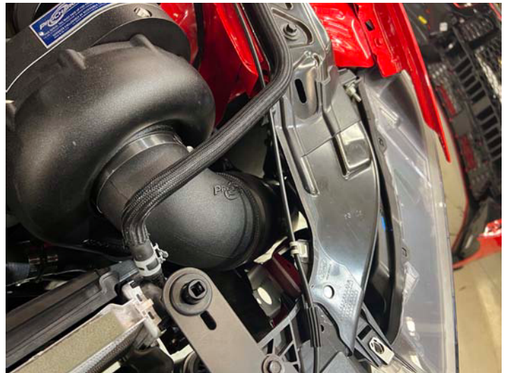
Rotomold Inlet Installed
