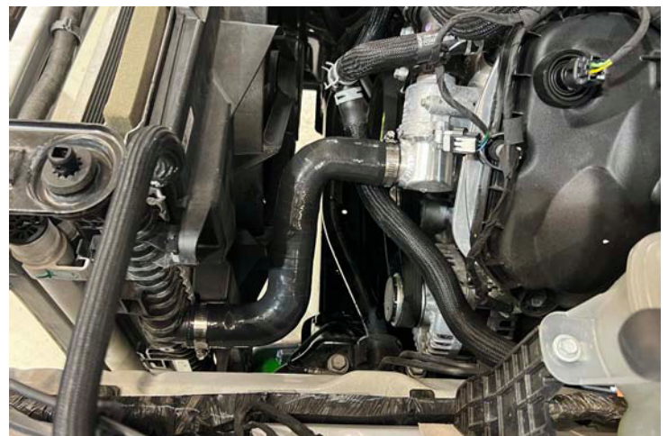
Lower Radiator Hose Installed
