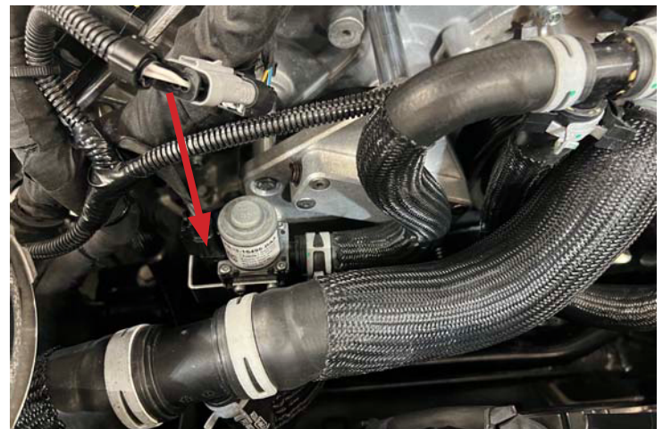
Coolant Solenoid Bracket installed
