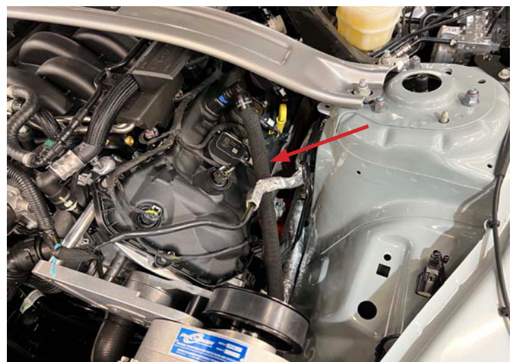
PCV Line Installed
